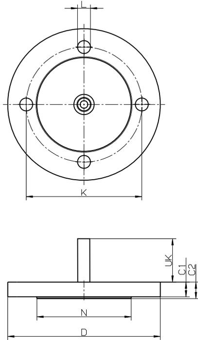
Alignment cable gland between flange holes
