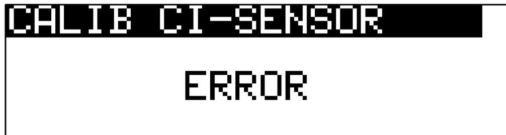
The calibration process must be terminated by pressing the
