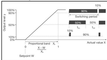
If actual value X exceeds setpoint W, the P controller will control in proportion to the control deviation. When the proportional band is exceeded, the controller operates with an output level of 100 % (100 % clock ratio).
