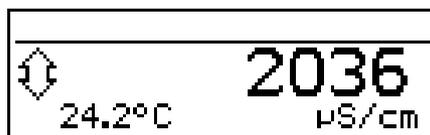
Here the numerical value is supplemented by a symbol to indicate the direction and speed of change for the measurement.
