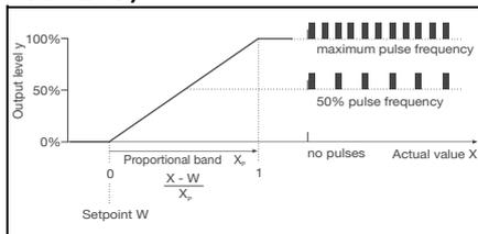
If actual value X exceeds setpoint W, the P controller will control in proportion to the control deviation. When the proportional band is exceeded, the controller operates with an output level of 100 % (maximum switching frequency).
