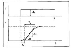
Example: calculation of the control parameters for a controller with PID action
