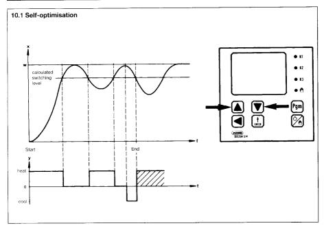
The controller is supplied as standard with self-optimisation (referred to below as SO) of the controller parameters.
