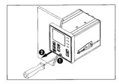
3 Lift the clips at the back and pull off the back panel
