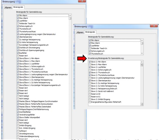
All fault messages are OR-linked and output as a binary signal for a collective fault on the relay output or optocoupler.
