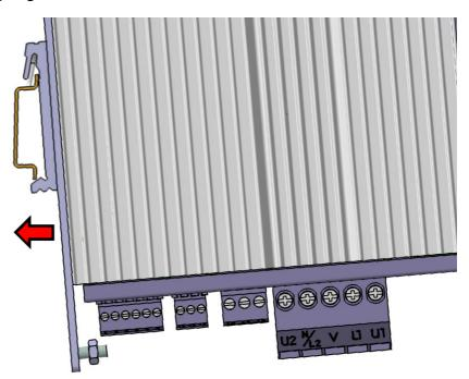
\* Swivel the power controller downward until the detent lug engages with the DIN rail with an audible click.
