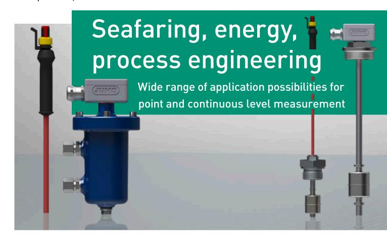
ith the product series NESOS, it is the first time that JUMO has brought to market devices for point level measurement using floats and reed contacts, and for level measurement using floats and reed chains. In these devices, a float with an integrated magnet uses its magnetic field to switch one or more reed contacts with rising or falling levels. The
