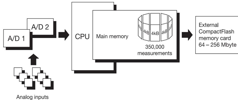
The measurements from the analog inputs are acquired continuously in a 250msec sampling cycle, and then stored in the main memory. These measurements also serve as the basis for limit monitoring.
