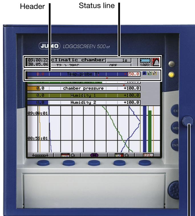
To open or close the door of the instrument, turn the knob
