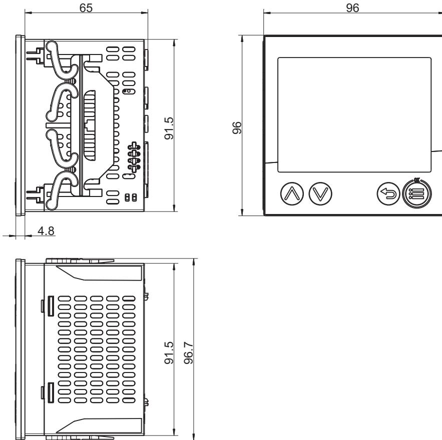
**Panel cut-out according to DIN IEC 61554**
