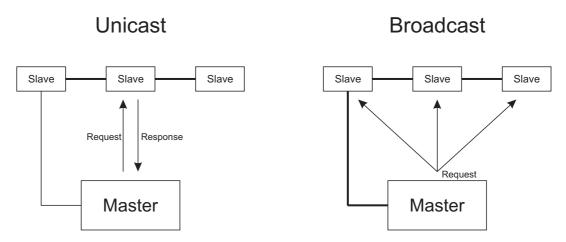
The master controls data exchange by cyclically querying the slaves on the overall bus. The slaves (e.g. JUMO ecoLine sensors) only have a response function. The master has write and read access to the slaves. This enables data to be communicated between master and slave devices in real-time. Slaves cannot communicate with one another directly. In order to transmit data from slave to slave, the master must extract data from one slave and transfer it to the next.
