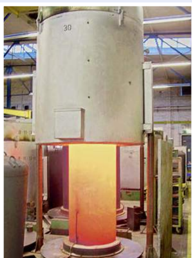
Bell furnace after removal of the heating mantle to start the cooling phase
