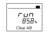
During deletion of the memory, a progress indication appears. If automatic data logging was active when the "Delete" function was started, it is ended. The instrument is "ready to measure" (REC blinks in the display).
