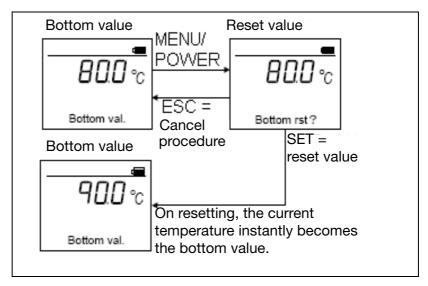
After SET or ESC, the display returns to showing the bottom value.
