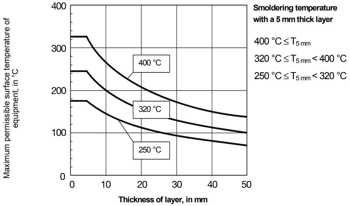
Figure 2: Reduction of the maximum permissible surface temperature with increasing thickness of the dust layer
