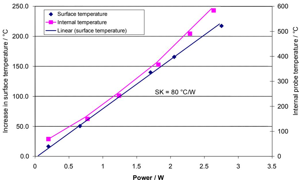
**Figure 1 : Self-heating of a Pt100 RTD temperature probe**
