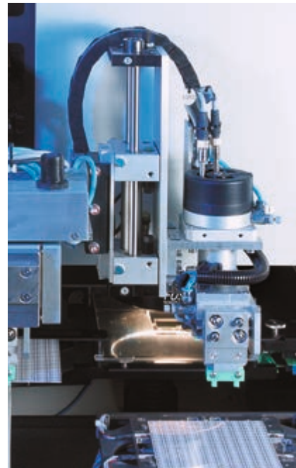
Laser trimming of platinum- chip temperature sensors
