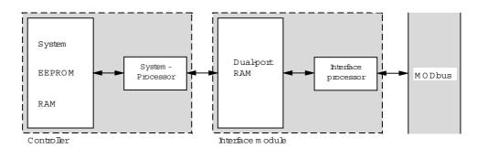
For data transmission to the MODbus, the system processor places the process values in a dual-port RAM. Not all the system variables which are present in the controlller are cyclically refreshed in the dual-port RAM. The dual-port RAM is divided into two areas:
