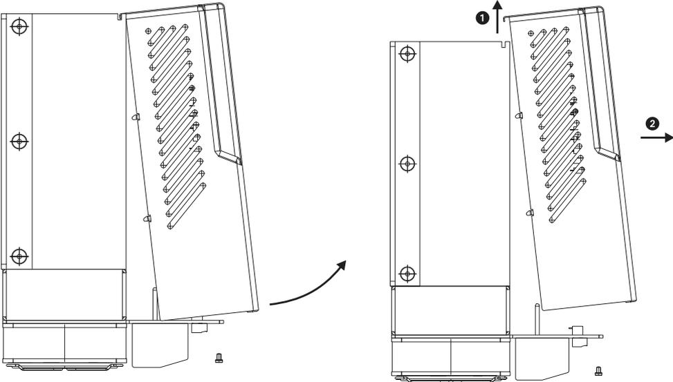
\* Lift the cover out of the groove ① and take it off forward ②
