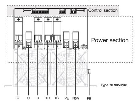
\* Make the connections to the screw terminals only with cables that have a suitable cross-section and are fitted with cable lugs.
