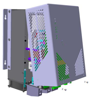
\* Lift the cover out of the groove 1 and take it off forward 2
