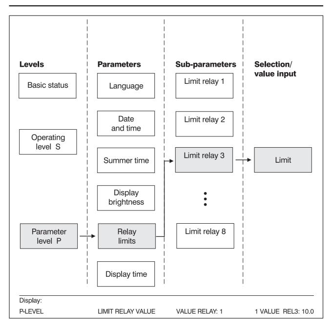
The levels, parameters and subparameters are arranged in a tree structure. Starting from the basic status the program branches to the individual levels and from there into the corresponding parameters, and also into any sub-parameters.
