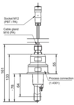
Split version for process connection 690 SMS 2' (union nut not included in delivery)
