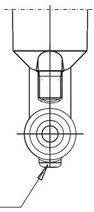
Extra code /268: temperature probe located internally
