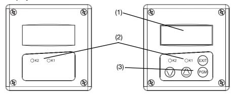
Version without a display Operation/configuration through the setup program only Version with a display Operation/configuration from the keys or through the setup program
