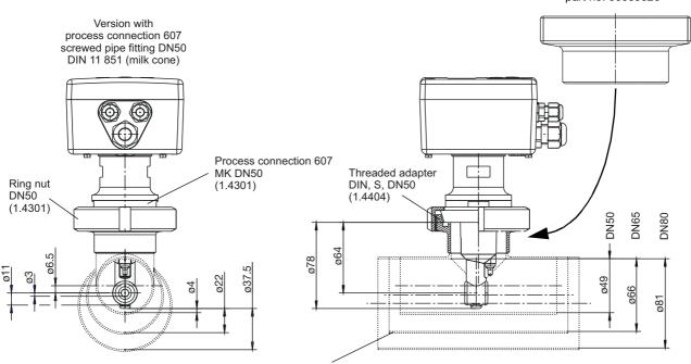
Reducing tee (to be provided by plant operator; <u>not</u> supplied by JUMO) DIN, short, SSS, DN50/50, DN65/50, DN80/50 (1.4301)
