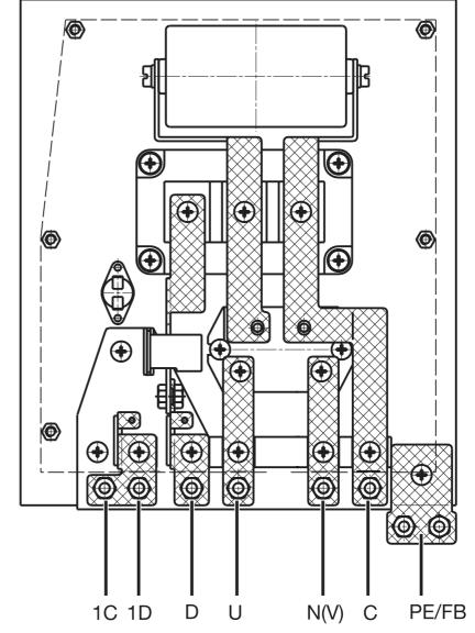
Make the connections to the screw terminals only with cables that have a suitable cross-section and are fitted with cable lugs. Maximum tightening torque 15 Nm.
