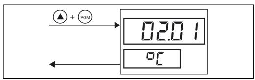
★ Display the software version and unit for temperature with ▲ + (mu)
