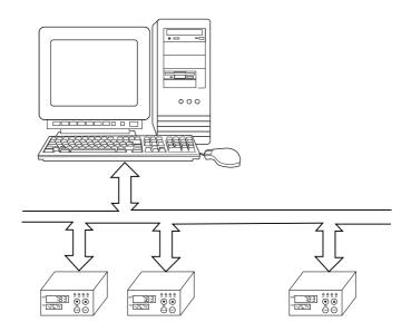
The bus system is designed around the master-slave concept. A master computer can communicate with up to 31 controllers or other devices (slaves). The interface is a serial interface using the RS422 or RS485 standards.
