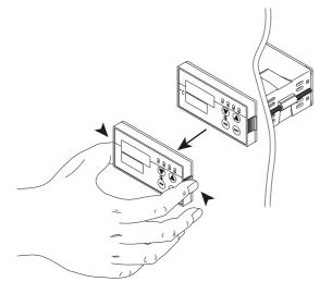
The controller module can be removed from its housing for servicing.
