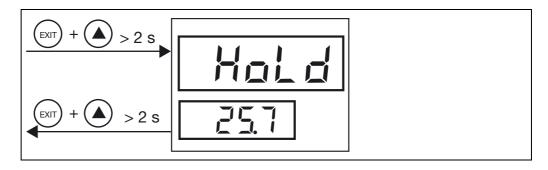
\* ( ) Press + ( for longer than 2 seconds (but less than 4 seconds)
