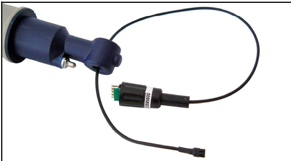
The calibration program will ask you to connect the first calibration resistor. The first calibration resistor is an open loop, as shown in the picture.
